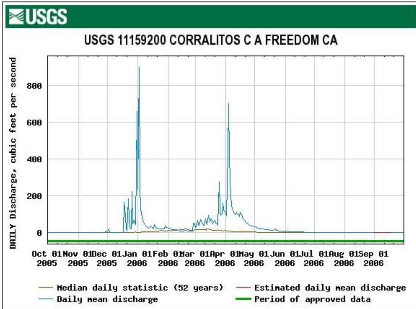
Figure 38. The 2007 Daily Mean and Median Flow at the USGS Gage on Corralitos Creek at Freedom. (USGS website would not provide a logarithmic scale of discharge).
