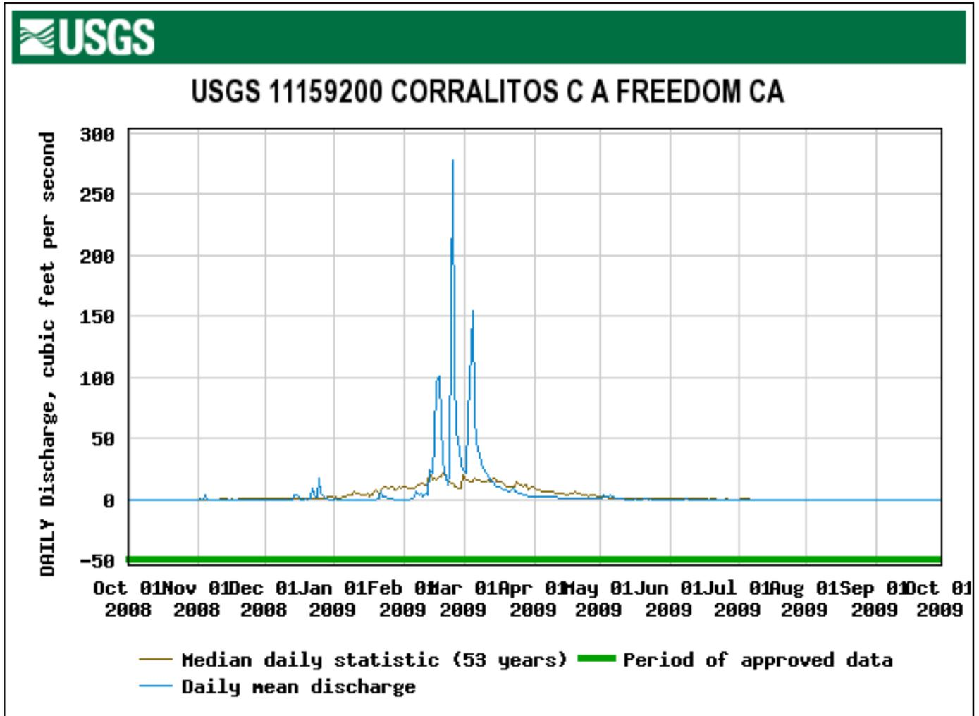
Figure 41. The 2010 Daily Mean and Median Flow at the USGS Gage on Corralitos Creek at Freedom. (USGS website would not provide a logarithmic scale of discharge).
