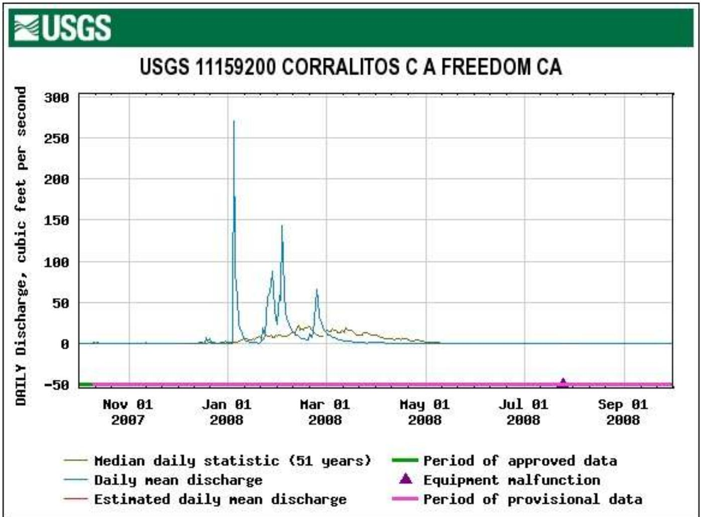
Figure 40. The 2009 Daily Mean and Median Flow at the USGS Gage on Corralitos Creek at Freedom. (USGS website would not provide a logarithmic scale of discharge).
