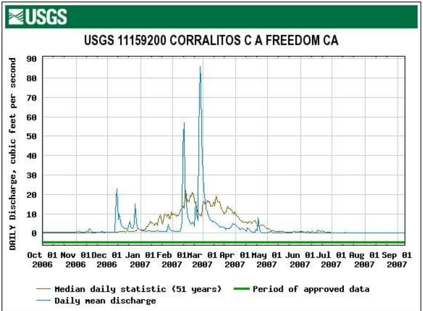
Figure 39. The 2008 Daily Mean and Median Flow at the USGS Gage on Corralitos Creek at Freedom. (USGS website would not provide a logarithmic scale of discharge).
