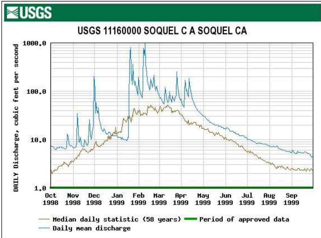
**Figure 23. The 2000 Daily Mean and Peak Flood Flow at the USGS Gage on Soquel Creek at Soquel.**
