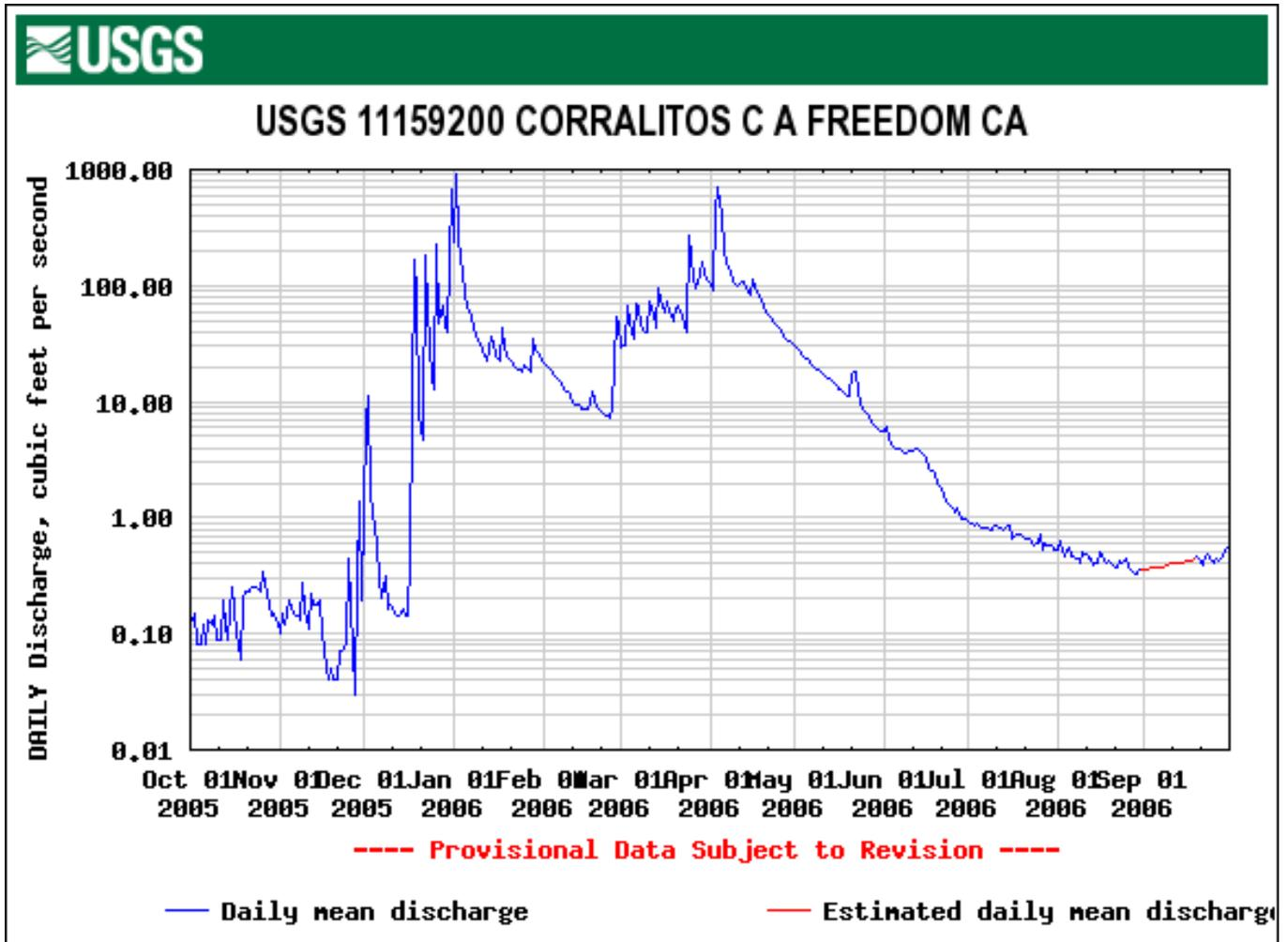
Figure 37. The 2006 Daily Mean Flow at the USGS Gage on Corralitos Creek at Freedom with Median Flow Statistics.
