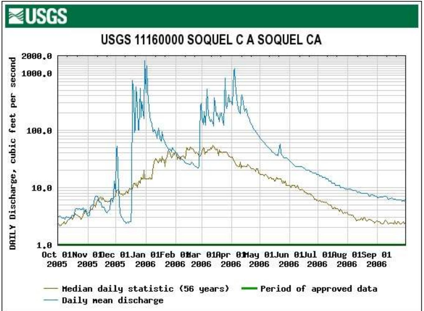
Figure 30. The 2007 Daily Mean and Median Flow at the USGS Gage on Soquel Creek at Soquel.
