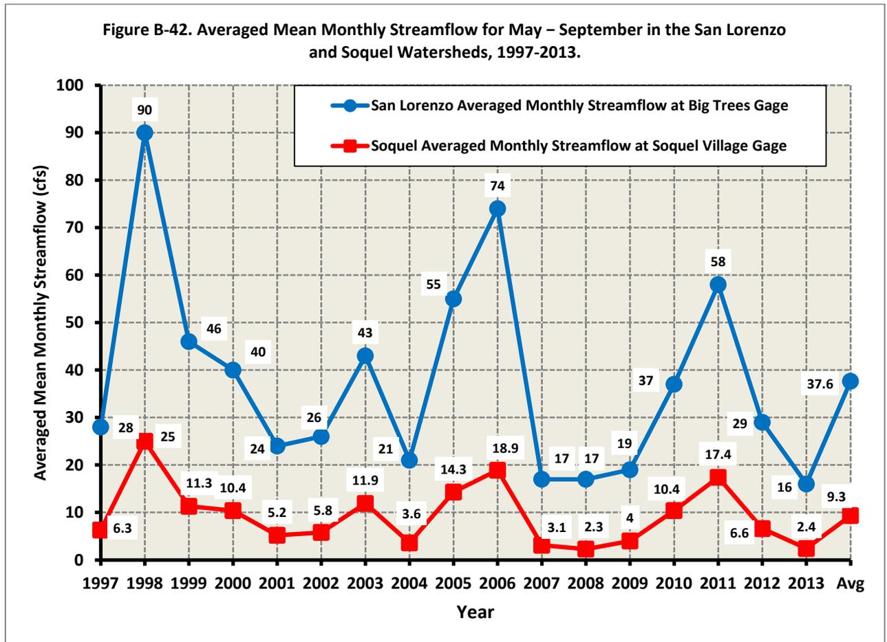
**Figure B-42. Averaged Mean Monthly Streamflow for May – September in the San Lorenzo and Soquel Watersheds, 1997-2013.**
