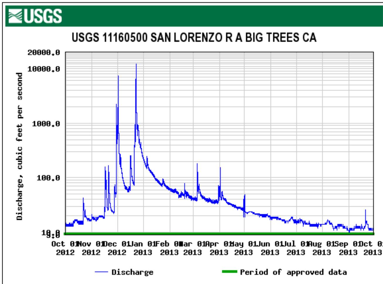
Figure B-34b. The 2013 Daily Average Discharge and Median Daily Flow of Record for the USGS Gage On the San Lorenzo River at Big Trees.
